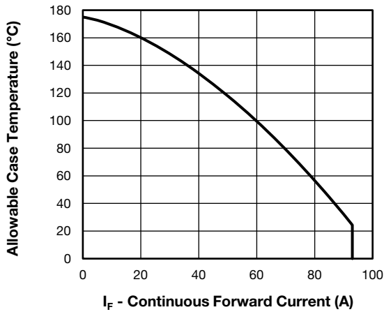
Fig. 3 - Maximum Allowable Case Temperature vs. Average Forward Current (Per Diode)
