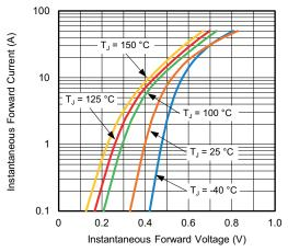
Fig. 3 - Typical Instantaneous Forward Characteristics
