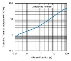
Fig. 6 - Typical Transient Thermal Impedance
