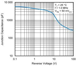
Fig. 5 - Typical Junction Capacitance
