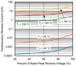
Fig. 4 - Typical Reverse Leakage Characteristics
