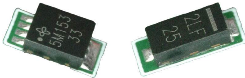
Real picture of DFN33A and DFN3820A after reflow soldering showing meniscus
