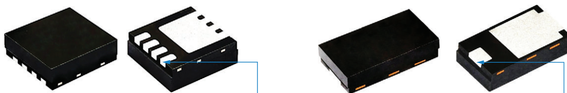
Wettable sidewall plated solder pads
