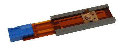
The interface features a low profile (thickness of 3 mm and width of 13.5 mm), allowing designers to take advantage of the performances of the UIPMA / UFPMA without having to manage the distance between the wiper and sensor surface. The pressure is auto-calibrated by the assembling performed in Vishay facilities.
