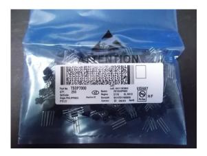
Be aware these counterfeit TSOP7000 devices do not function correctly. The parts shown above were shipped with lookalike Vishay mailing labels and packing boxes. Vishay obtained samples from this lot and determined beyond any doubt that the devices are counterfeits.
