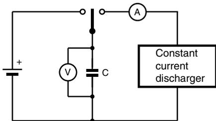
Fig. 4 - Test circuit for capacitance measurement
