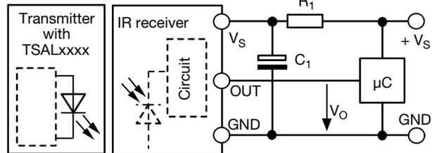
$R_1$  and  $C_1$  recommended in case there are strong ripple or spikes on the supply line.
