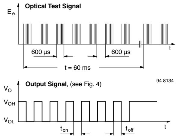
Fig. 3 - Test Signal
