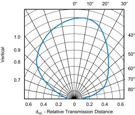
Fig. 11 - Horizontal and Vertical Directivity
