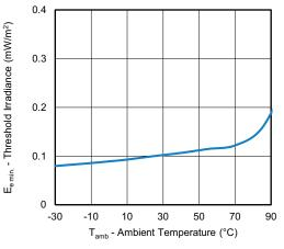
Fig. 9 - Sensitivity vs. Ambient Temperature
