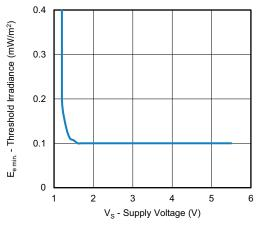
Fig. 12 - Sensitivity vs. Supply Voltage
