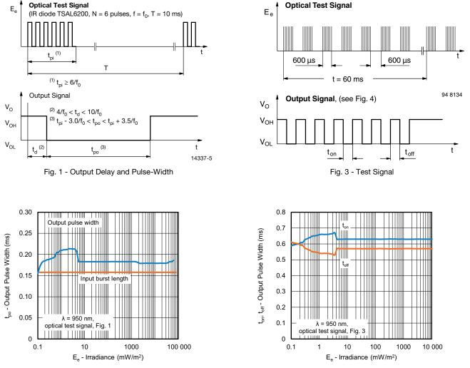
Fig. 2 - Pulse-Width vs. Irradiance in Dark Ambient
