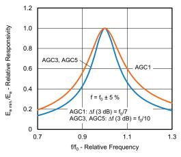
Fig. 5 - Frequency Dependence of Responsivity
