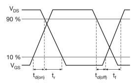
Fig. 19 - Waveforms of Switching Time
