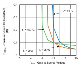
Fig. 12 - On-Resistance vs. Gate-to-Source Voltage
