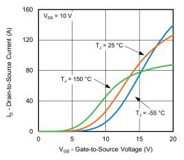
Fig. 4 - Typical Transfer Characteristics
