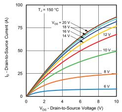
Fig. 3 - Typical Output Characteristics
