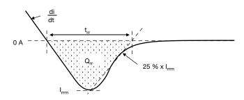
Fig. 23 - Waveforms for Reverse Recovery
