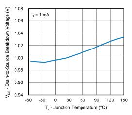
Fig. 10 - Temperature vs. Drain-to-Source Voltage
