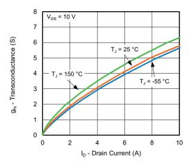
Fig. 5 - Forward Transconductance vs. Drain Current
