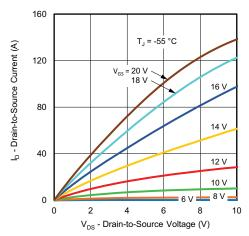
Fig. 1 - Typical Output Characteristics
