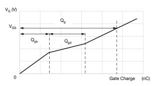
Fig. 22 - Waveforms for Gate Charge
