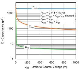
Fig. 7 - Typical Capacitance vs. Drain-to-Source Voltage
