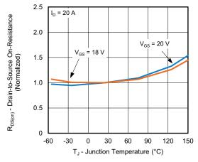
Fig. 9 - Normalized On-Resistance vs. Temperature
