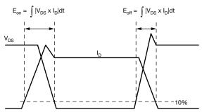
Fig. 20 - Waveforms for Switching Energy
