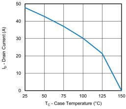
Fig. 14 - Drain Current vs. Case Temperature
