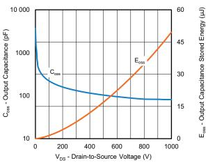
Fig. 15 - Output Capacitance and its Stored Energy vs. Drain-to-Source Voltage
