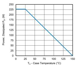
Fig. 16 - Power, Dissipated P<sub>D</sub> vs. Case Temperature
