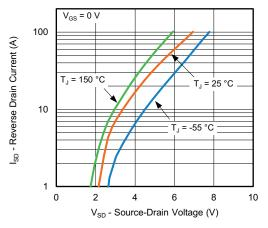
Fig. 11 - Typical Source-Drain Diode Forward Voltage
