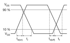
Fig. 19 - Waveforms of Switching Time
