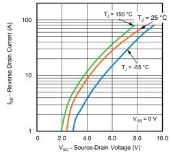
Fig. 11 - Typical Source-Drain Diode Forward Voltage
