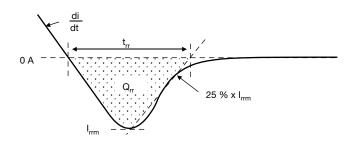
Fig. 23 - Waveforms for Reverse Recovery
