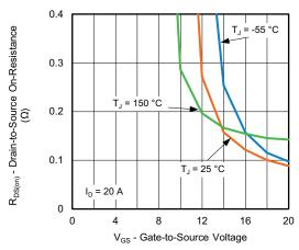
Fig. 12 - On-Resistance vs. Gate-to-Source Voltage
