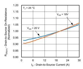
Fig. 6 - Normalized On-Resistance vs. Drain-to-Source Current
