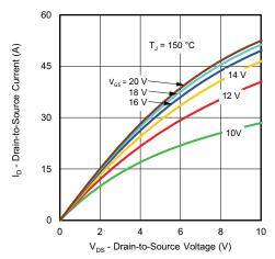
Fig. 3 - Typical Output Characteristics
