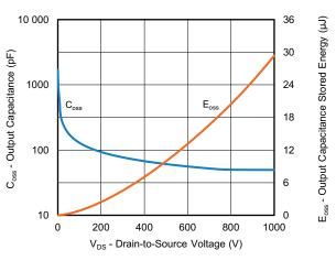
Fig. 15 - Output Capacitances and its Stored Energy vs.
