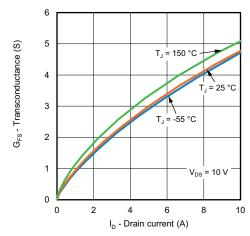
Fig. 5 - Forward Transconductance vs. Drain Current
