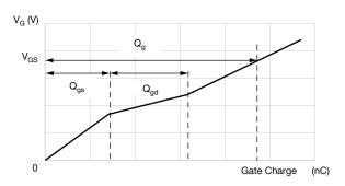
Fig. 22 - Waveforms for Gate Charge
