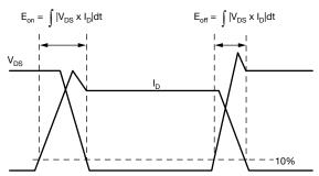
Fig. 20 - Waveforms for Switching Energy
