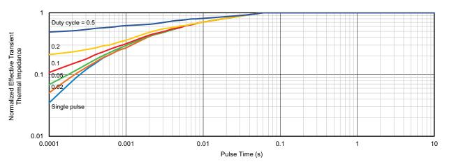
Fig. 18 - Normalized Effective Transient Thermal Impedance
