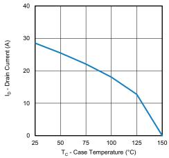
Fig. 14 - Drain Current vs. Case Temperature
