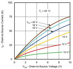
Fig. 2 - Typical Output Characteristics
