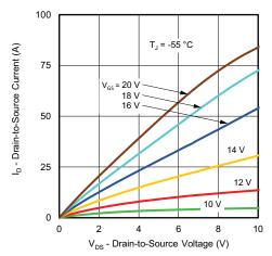
Fig. 1 - Typical Output Characteristics
