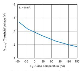
Fig. 13 - Threshold Voltage vs. Case Temperature
