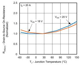
Fig. 9 - Normalized On-Resistance vs. Temperature
