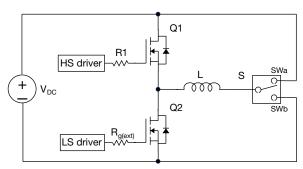
Fig. 21 - Switching and Reverse Diode Characteristics Measurement Circuit
