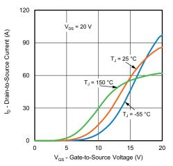
Fig. 4 - Typical Transfer Characteristics
